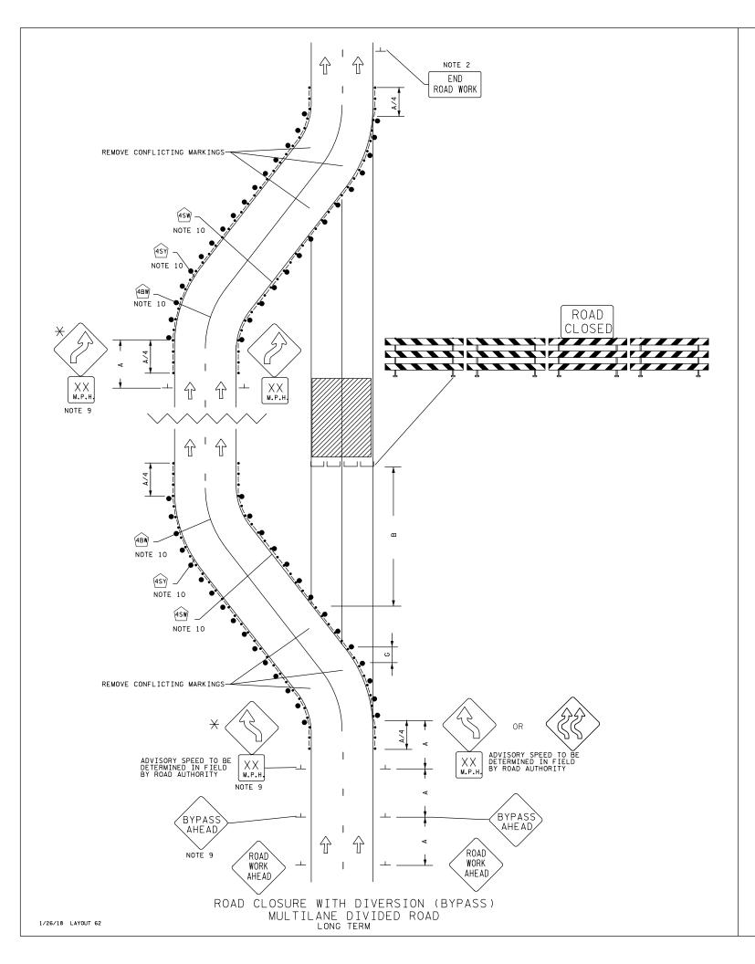
POSTED SPACI SPACING SPEED OF LIMIT PRIOR TO ADVANO CHANNEL IZ ING DEVICES WARNI WORK SIGNS (G) STARTING (A) (MPH) FEET FEET 0 - 30 100 25 35 - 40 325 45 - 50 600 750 55 50 1000 60 - 65 1200 70 - 75
